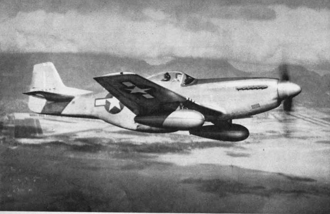
Veteran of Europe , the P-51 ( above ) bases on Iwo Jima for strikes against Japan. Angular in wing and tail, it has a curving back and belly line. Newest AAF fighter to reach the Pacific is the long-range P-47N ( below ). Note the squared-off wing and the long, low fin extension.
